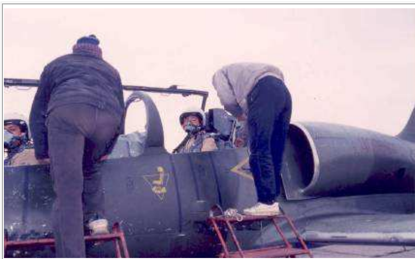
Ground crew checking oxygen hose and strapping me on to L-39
